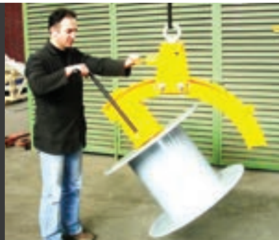
LIFTED "TILTER" TILTING THE REEL
