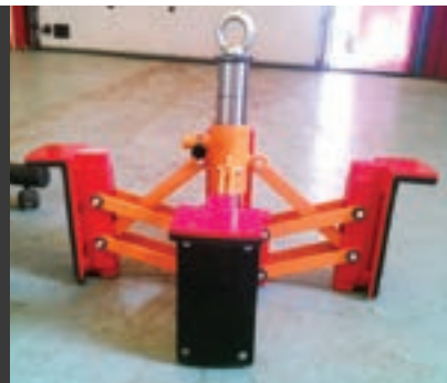
"LIFTER" TRANSPORTING THE COIL
