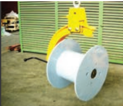
"TILTER" PLACED IN THE REEL BORE
