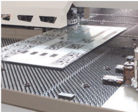
■ Brush and ball bearing type table facilitates sheet metal loading and unloading (S)
