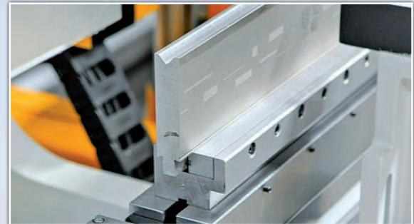
This system determines the order of use of the partial dies, which are mounted on the upper beam in full length, and attached to the top tool holder, by means of laser beam.
