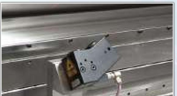
Developed by Data M Engineering, it is a powerful solution for measuring bending angles in press brakes.
